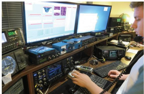
Most of the antennas here are mono band, so no ATU is needed, however, one low band antenna had a slightly higher SWR and this caused the amp to get a little hotter hence hearing the fan.
